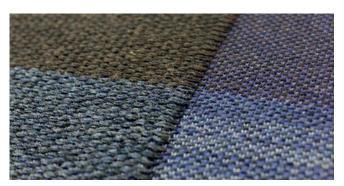
Material combinations of heavy-count yarn integrated into a fine structure.
