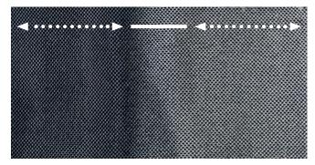
Integration of thermo-fusible yarns for sectional reinforcement and shape stabilization.
