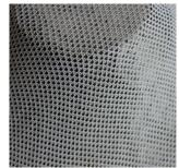
Weft-reinforced fabrics using carbon fiber materials.
